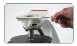
2. Align the shape of the module with the shape of the microscope stand.
